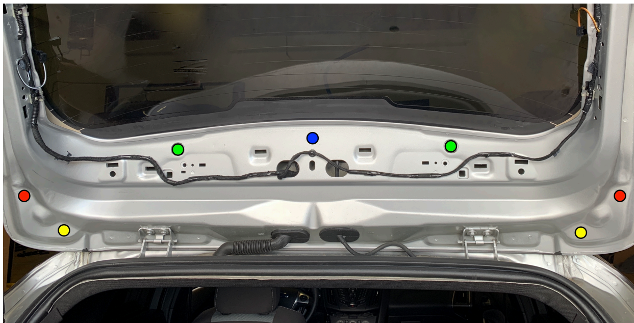
FIGURE 2 - WING FASTENER + STANDOFF LOCATIONS (INSIDE OF TAILGATE PICTURED, WITH PLASTIC TRIM REMOVED)
