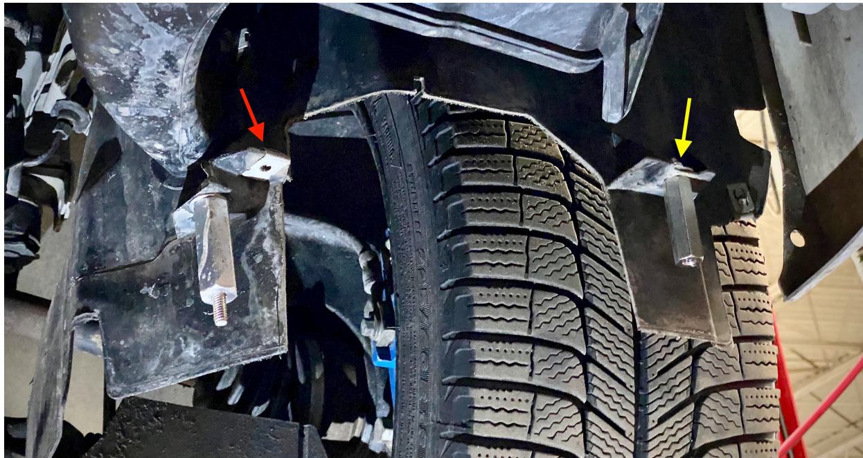
FIG. 4 - RED ARROW= OEM SCREW; YELLOW ARROW= STANDOFF LOCATION
